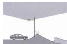
Poorly directed parking lot lighting
