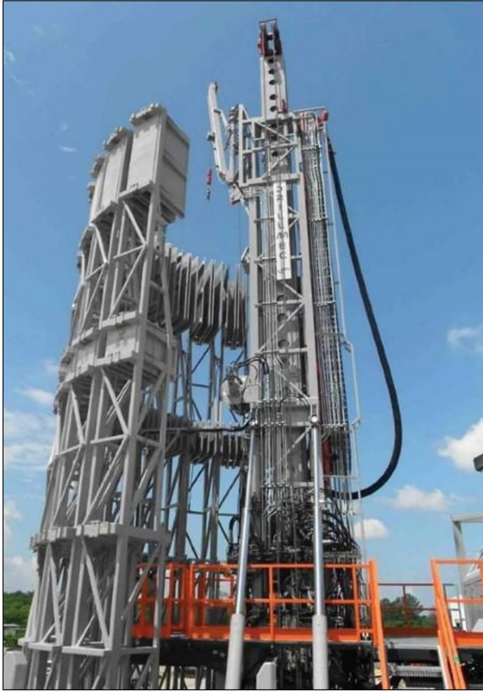
Figure 3.4-1 Example Drill Rig for a Slim-hole Well
